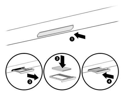
To remove the SIM card, press in gently on the SIM card access tray to disengage the SIM lock, and the tray will pop out of the slot. Remove the SIM card. Replace the tray in the computer and press in gently on the tray until it is firmly seated.
