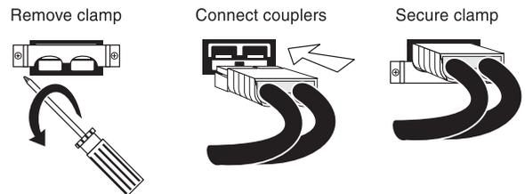
1. Use a phillips screwdriver to remove the battery pack coupler clamps from the UPS and from all but the last Battery Pack.
