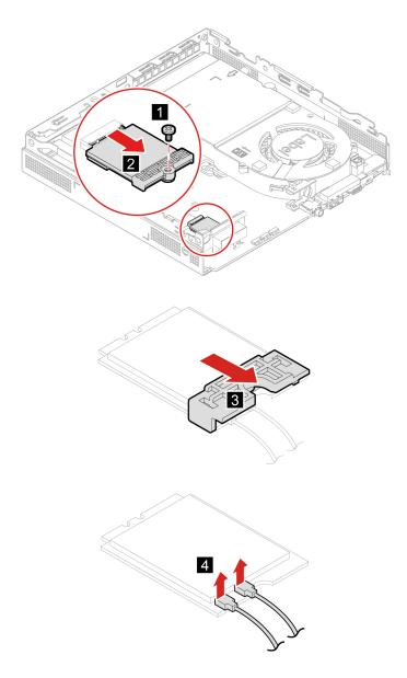
Note: While installing, ensure that you connect the gray cable to the connector labeled 1 (auxiliary) and the black cable to connector labeled 2 (main) on the card.
