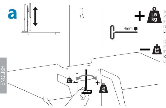
Increase Lift Strength If the mounted weight is too heavy or this product does not stay up when raised, then you'll need to increase Lift Strength:
