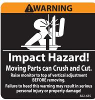
Warning: Impact Hazard! Moving Parts can Crush and Cut. Raise monitor to top of vertical adjustment before removing.
