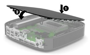
2. Insert the hooks on the left side of the rear I/O panel (1) into the left side of the back of the chassis, rotate the right side (2) to the chassis, and then press the right side into the chassis until it locks in place.
