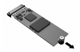
5. Pull the screw kit off the storage module and attach it to the replacement storage module.
