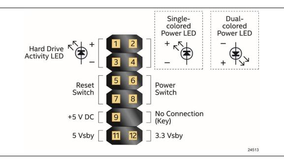
Figure 10. Connection Diagram for Front Panel Header (2.0 mm Pitch)
