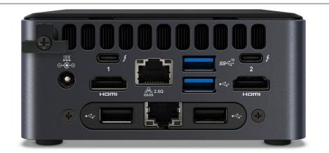
Figure 16. Dual LAN Chassis Image Back Panel
