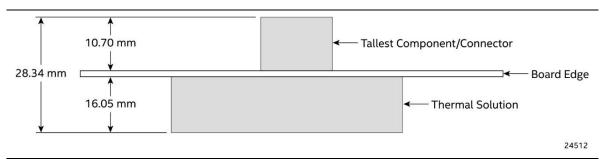
Figure 21. Board Height Dimensions
