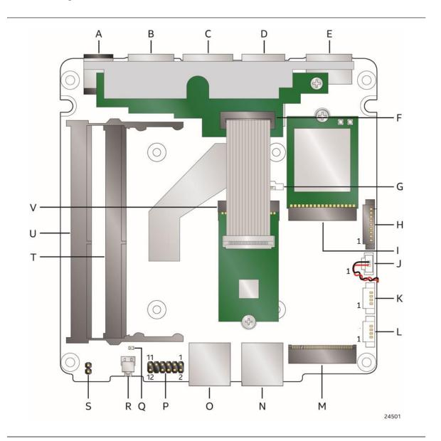
Figure 2. Major Board Components (Dual LAN only) (Bottom) with Pin 1 Indicators
