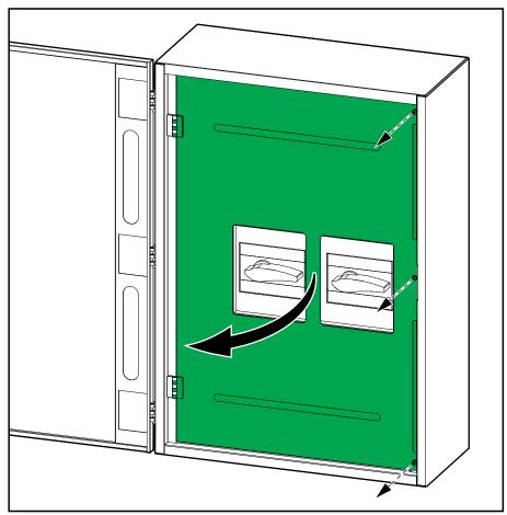
4. Mount the parallel maintenance bypass panel to the wall.
