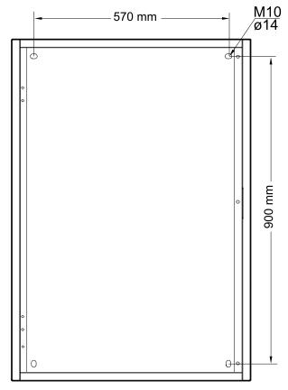
2. Drill holes in each of the four marked locations and mount the anchor bolts.
