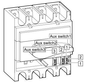
2. Connect signal cables (not supplied) from the three AUX switches in the maintenance bypass switch MBB to the UPSs.
