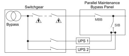
The upstream disconnection switchgear must be suitable for disconnection purposes. Before working on the upstream supply, the MBB must be locked in the open position using the built-in lockout function.
