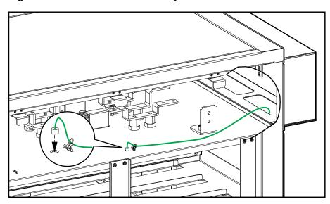
7. Route the battery temperature sensor cables through the conduit box to the UPS. Disconnect the cables from J2–1 and J2–2 and connect the battery temperature sensor.
