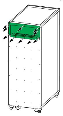
2. Rotate the conduit box and install.
