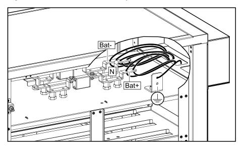
5. If more than one modular battery cabinet is part of the installation, connect the battery cables (kit E3MOPT006) between the modular battery cabinets.
