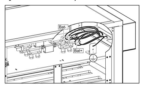
5. If more than one modular battery cabinet is part of the installation, connect the battery cables between the modular battery cabinets.
