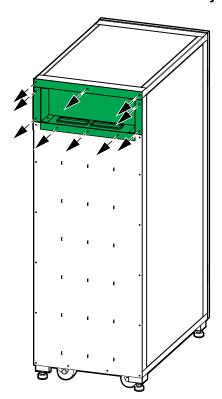
2. Rotate the conduit box and install.
