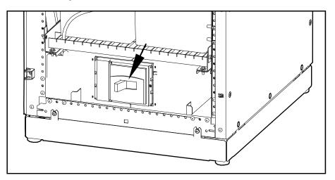
11. Disconnect all battery units by removing them (all battery types) or pulling them out to the disconnect line (modular batteries only).
