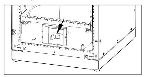
Set the SYSTEM ENABLE switch on the UPS to the ON position.NOTE: Wait approximately two minutes for the system to start.
