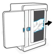
4. While holding onto the blue latch, align and insert the panel as shown. Release the blue latch to lock the panel in the place.
