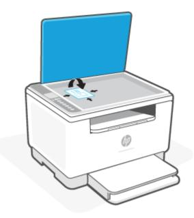
4. Close the scanner lid and press (1) (the Resume button) to start scanning the second side and print.
