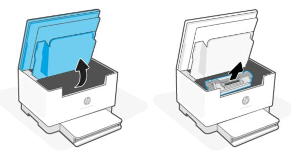
2. If you can see the jammed paper, carefully grasp the jammed paper, and slowly pull it out of the printer.
