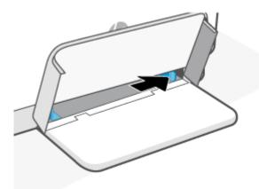
3. Insert the stack of paper into the input tray with the top forward and the side to be printed on facing up.
