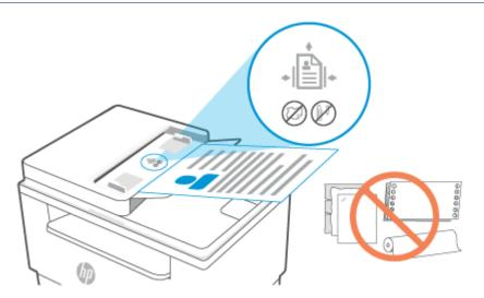
2. Slide the paper-width guides inward until they stop at the left and right edges of the paper.
