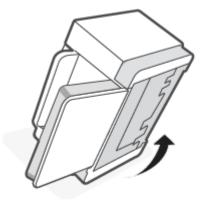
5. Release and hold on to the blue latch, and then remove the panel.
