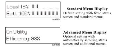
**Note:** The standard menu is the default setting and does not contain all of the menus and attributes of the advanced menu. The advanced menu automatically scrolls through multiple screens.
